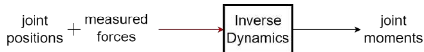
Figure 17: Parameter estimation for dynamic model. Inverse dynamics is used to compute joint moments from joint positions and measured forces.
