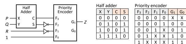
The circuit above may be replaced by a single 2-input logic gate. Choose the logic gate from this list: OR, AND, NOR, NAND, XOR, XNOR.
