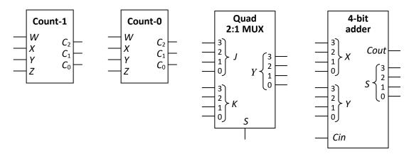
Given the above 4 components, you are to employ block-level design to design the converter, <u>without</u> <u>using any additional logic gate or other devices</u>. You may observe that if A = 1, then the output *FGH* is simply the number of 1s in the input *ABCD*. You are to make your own observation for the case when A = 0.
