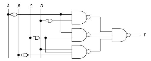
Students: Draw logic diagrams neatly with straight lines. Draw thick dots to represent forks.
