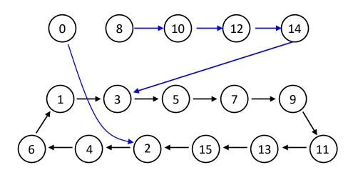
The circuit is self-correcting as any unused state can transit to a used state after a finite number of cycles.
