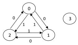
A circuit is **self-correcting** if for some reason the circuit enters into any unused (invalid) state, it is able to transit to a valid state after a finite number of transitions. Is your circuit self-correcting, and why?
