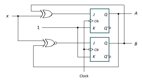
After committing the expressions for the flip-flop inputs, the don't-care values below are replaced with actual values (in parentheses). The state diagram with the unused state 3 is shown below. It is a self-correcting circuit, since there is an arrow out from state 3 to a used state.
