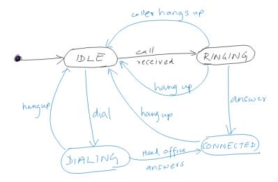
Note that it is assumed that the phone does not go from CONNECTD to IDLE unless the 'HANGUP' button in pressed, even if the phone at the other end was hung up.
