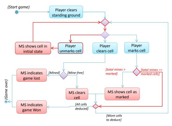
Note that some actions/paths have been deleted. The above diagram uses a diamond as either a branch or a merge (but not both). It is ok to use a diamond as both a merge and branch, as long as it does not lead to ambiguities.
