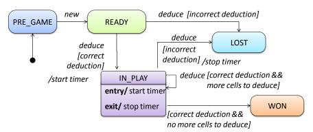
However, the above SMD does not give the desired behavior because the *deduce* event triggers both entry and exit activities every time a new cell is deduced! That means the timer will start from zero every time a cell is deduced. To rectify this, it can be made an internal activity, as shown below.
