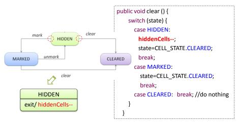
When superstates are involved, all the sub-states are simply grouped together in the switch statement. Note that the switch statement does not have a separate case for the superstate. Neither are superstates declared as a member of the enumeration.
