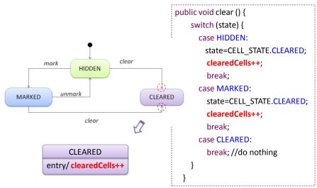
Similarly, exit activities are inserted where the state variable is changed from the state in concern (i.e. the one that has the exit activity) to another state. The example below shows how the HIDDEN state's exit activity is inserted into the clear() operation. Note that according to the SMD, there are two ways to exit the HIDDEN state (clear() operation and the mark() operation), both of which need to incorporate the exit activity.
