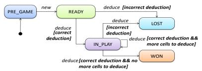
An *activity* is a behavior that takes place *during* a transition. The UML syntax is event[guard]/activity where all 3 components are optional. Note that in the context of SMDs, 'activity' 'action' and 'effect' are used interchangeably. In the following SMD, it is assumed that MS keeps track of the time taken for a game.
