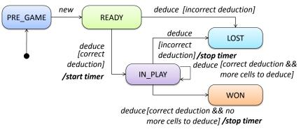
Alternatively, the start timer and stop timer can be included as *internal activities* in the IN\_PLAY state. An *entry activity* is an internal activity that is executed whenever object enters the state. Similarly, the *exit activity* is an internal activity that is executed whenever object exits the state.
