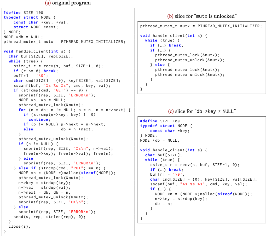
Fig. 1. An example program (a) that implements a simple key-value server. The example program includes an unbounded loop ( while (true) ... ), interaction with the external environment ( recv/send ), and heap manipulating data-structures ( NODE ). In addition, slices (b) and (c) corresponds to the post-conditions “ mtx is unlocked” (always holds) and “ db->key ≠ NULL ” (may not hold) respectively.
