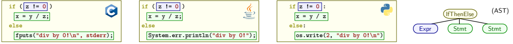
Fig. 5. Example AST representation of an if-then-else statement across the C, Java, and Python programming languages. Each AST node is represented generically by the file range from which the element was parsed, as illustrated by the nested colored boxes.
