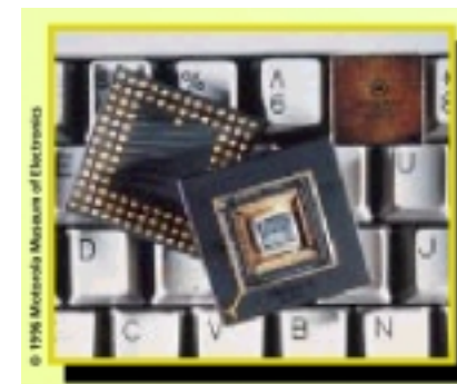
© 1996 Motorola Museum of Electronics 1984 Motorola introduces the MC68020 with 250,000 transistors.
